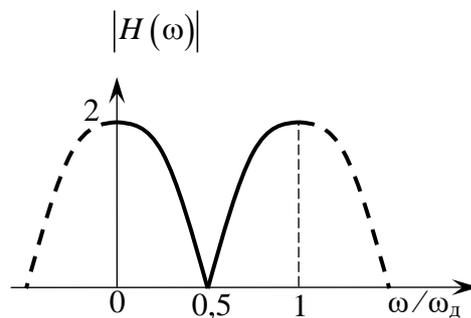
$$\varphi(\omega) = \begin{cases} -\omega\Delta t/2, & 0 \leq \frac{\omega}{\omega_d} < 1/2 \\ \pi - \omega\Delta t/2, & 1/2 \leq \frac{\omega}{\omega_d} < 1 \end{cases}$$
